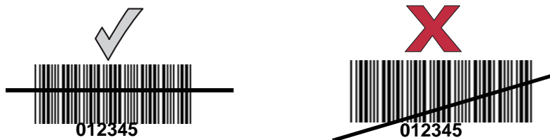
Figure 2-3 Acceptable and Incorrect Aiming
